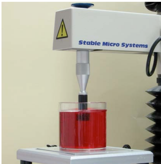
Abb. 4: Texture Analyser TA-XT2i
