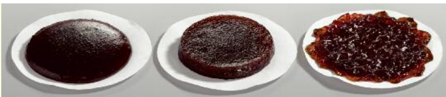
Fig. 5: Baking test 3 (left to right limited baking stable, baking stable, not baking stable)
