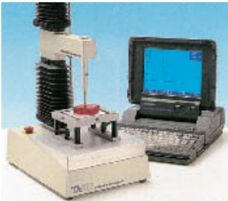
*Texture Analyzer for determination of gel strength*
